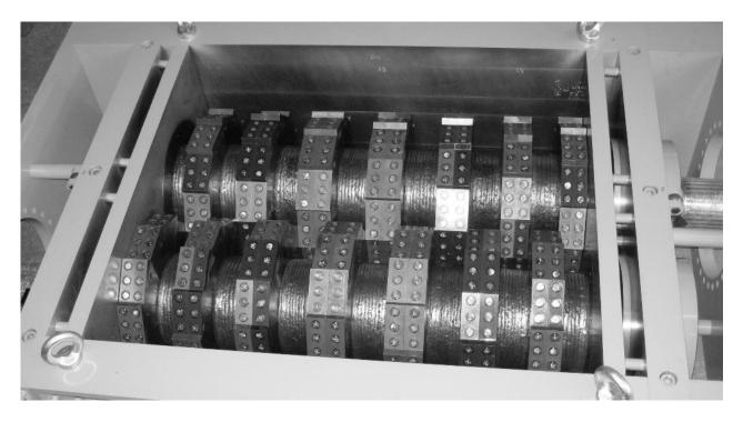
The main advantage of this shredder is, that knives are easy changeable without dismounting the shredder and the price for spare parts (operating costs) is much lower then in common shredders. After aprox. 6 000 t it's necessary to turn the knives. After another 6 000 t knives have to be sharpened. Because shredder has 4 different size of knives (105, 95, 85 and 75 mm) only 96 pcs knives size 105 mm should be added and the others are sharpened to smaller size (105 to 95 and so on).
